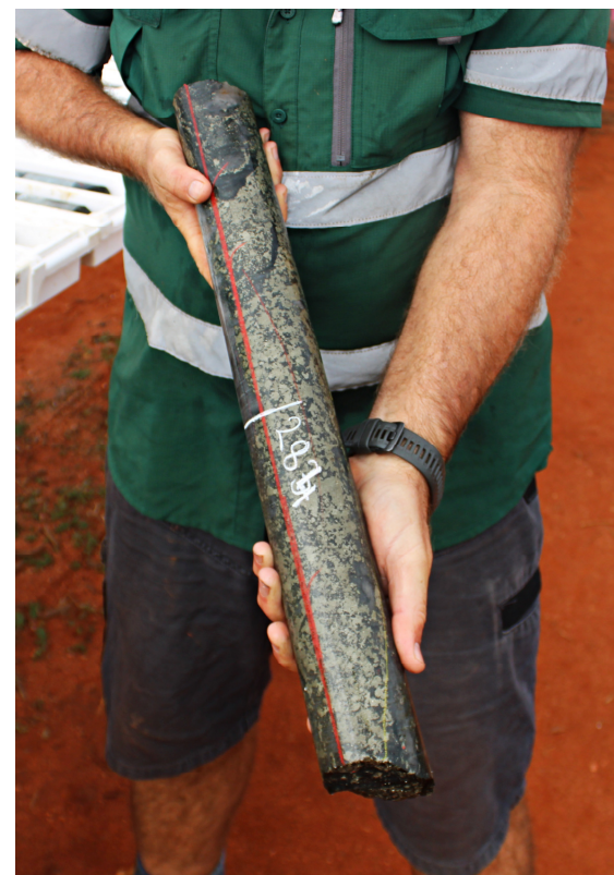
Figure 1: BHD026 core from 283.7 to 284.4m showing massive sulphide through altered Gabbro
