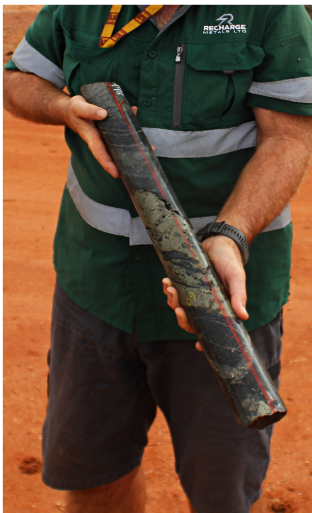
Figure 5: BHD026 core from 198 – 198.8mm, showing blebby sulphides through altered ultramafic
